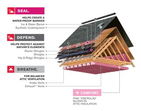
††† Use of shingle-over ridge vents will affect the impact resistance classification of the ProEdge Storm\* Hip & Ridge Shingles; use off-ridge ventilation as an alternative. Refer to the installation instructions for complete details.
